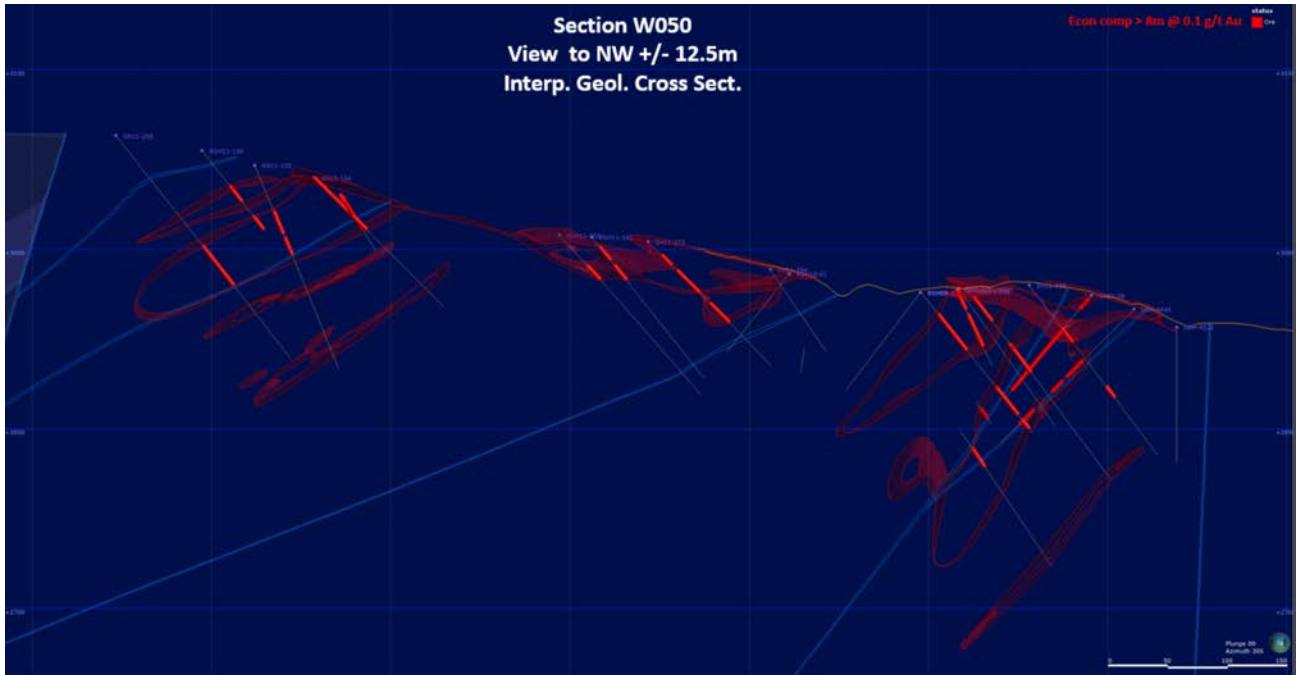
Figure 12.3 Grade shell - solids vs. drillhole gold assay composites
