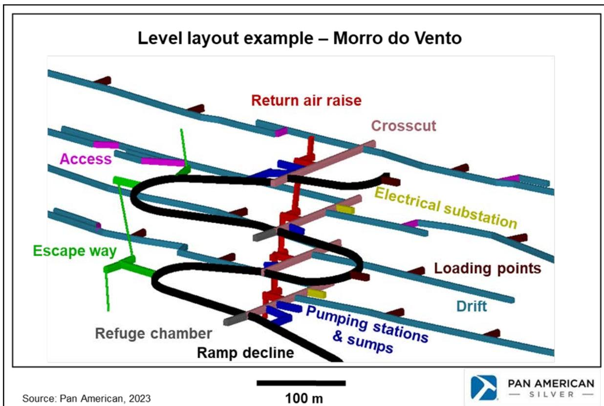
Figure 15-1: Level layout example
