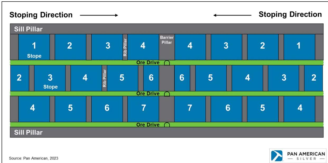
Figure 16-1: Example of typical mining sequence
