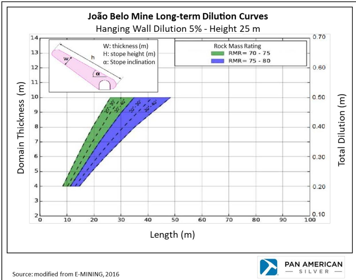
**Figure 16-5: Stability chart with dilution curves**
