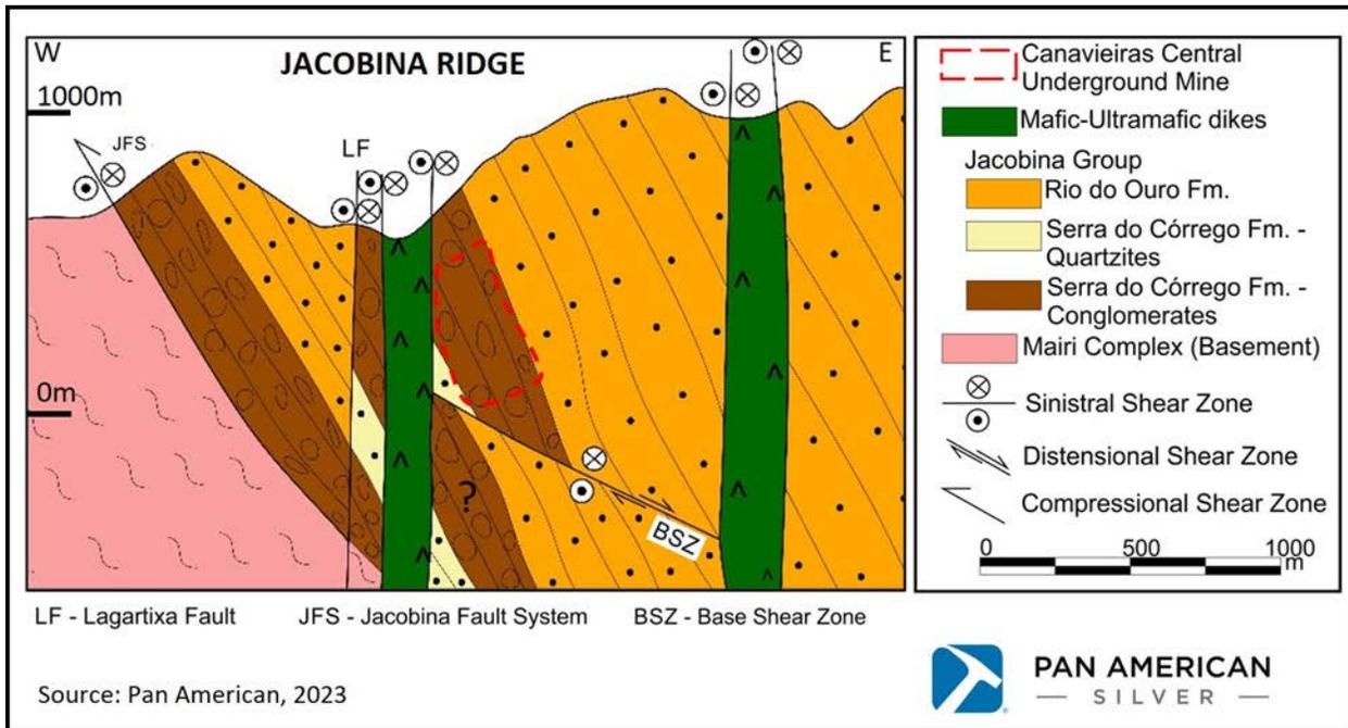
Figure 7-6: Generalized cross-section through the Canaveiras Central Mine
