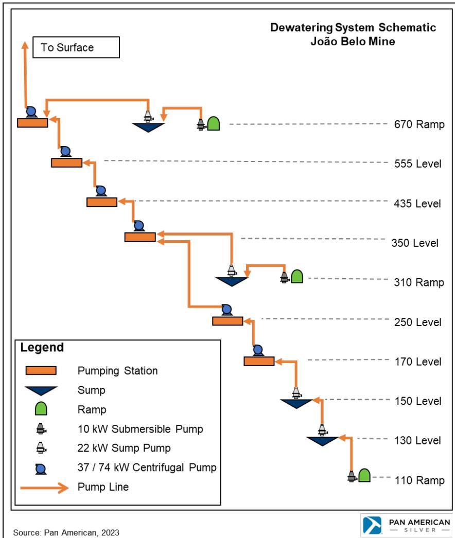
Figure 16-10: Schematic drawing of dewatering system at João Belo Mine
