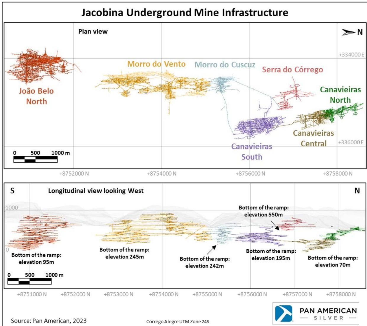
Figure 14-1: Plan (top) and longitudinal view (bottom) of the mine infrastructure
