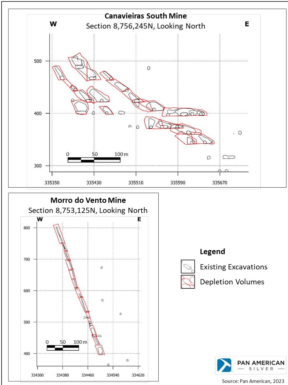
Figure 14-2: Example of excavation and depletion models at Canavieiras South and Morro do Vento mines
