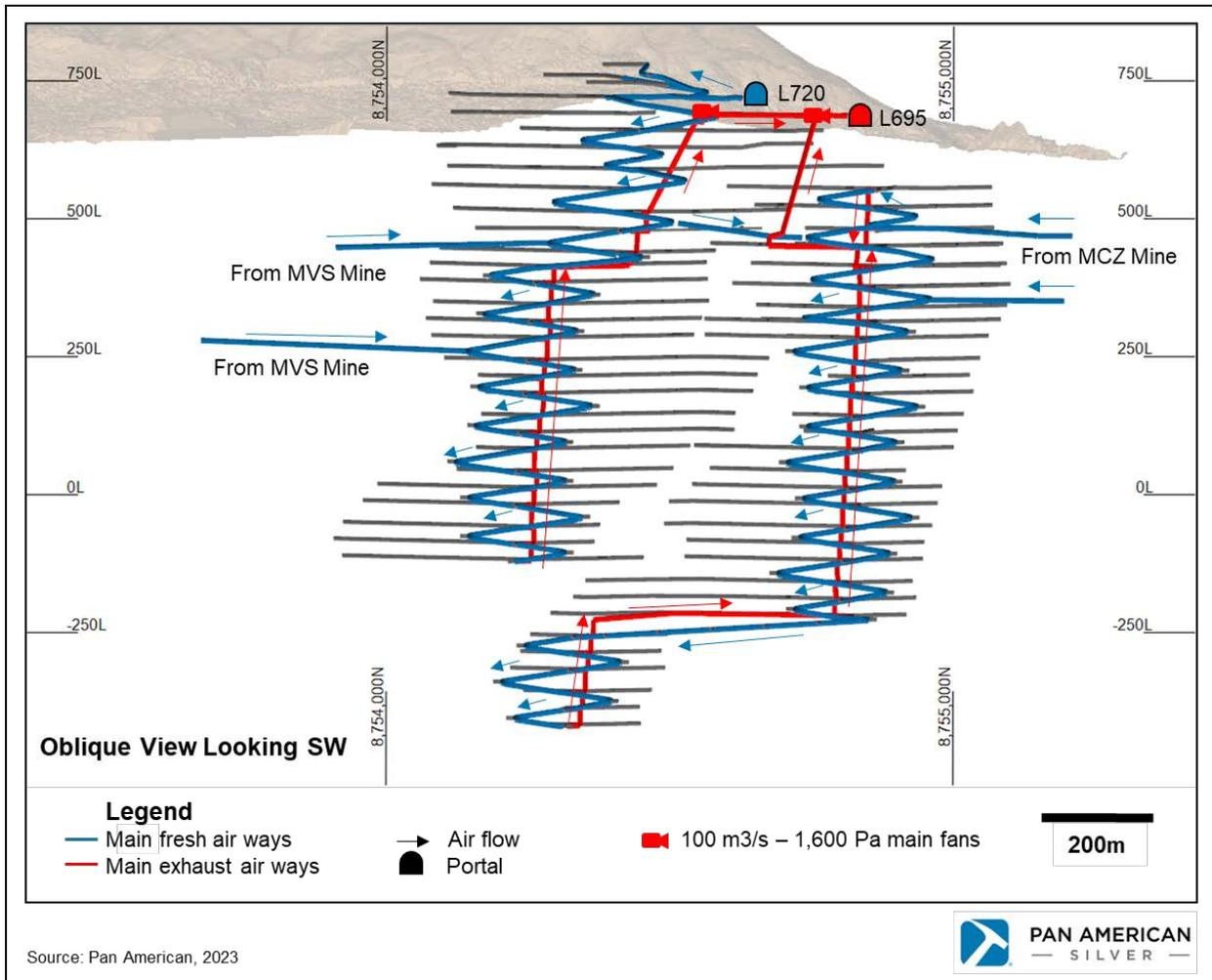
Figure 16-9: Schematic view of ventilation circuit - Morro do Vento Central Mine
